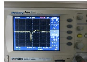
Speaker generates back electromotive force (EFM), disturbing accurate drive.
