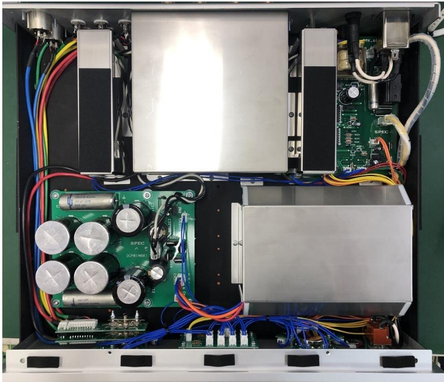
The R-core transformer and other components are separated by a shielding structure. In addition, EMC coating is applied to the inner surface of the chassis, reducing internal electromagnetic noise.
