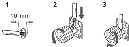
The connection terminals on this product are also compatible with Y lug terminals and banana plugs.
