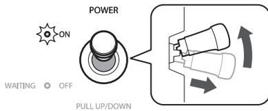
Check that the ON indicator on the body front panel is lit.
