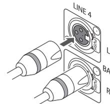
When disconnecting an XLR plug, press the latch lever (the part with "PUSH" inscribed on it) while pulling the cable. Use caution, as forceful disconnection may damage the unit.
