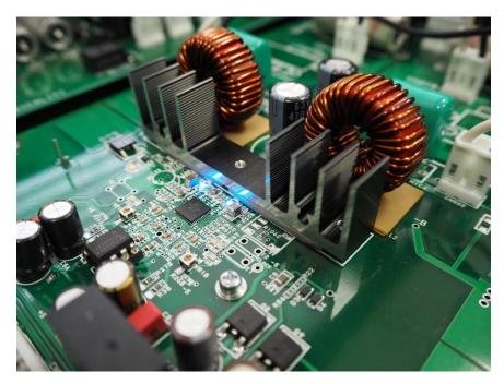
The Class D FET (under the heat sink) and the low pass filter placed very close to the FET.
