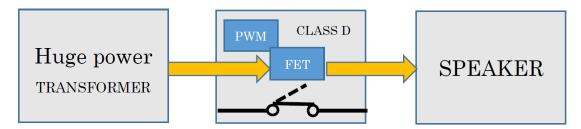
Very small FETs by Infineon Technologies supplies powerful energy directly to the speakers reproducing the sound pressure of the instrument. That's because Class D works just as a switch instantaneously. Sound pressure is the energy of the instrument itself. Additionally, simple and small circuit enables the sound with high-speed and highly clear tone. This is possible due to FETs almost completely preventing heat generation. There is no huge heat sink. Only a small heat sink is on the board.
