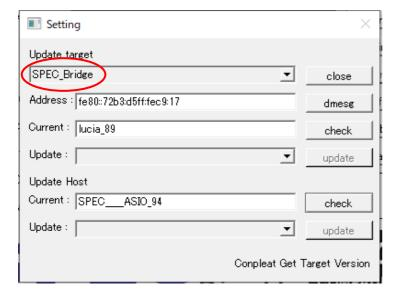
5: If you click "Check" and there is new firmware, a display different from the current display (the one with a large value of lucia\_xx) will be displayed in the Update section.
